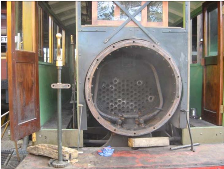
**(Above) No, its not a 38 class smoke-box but tube replacement still entails hard work.**
