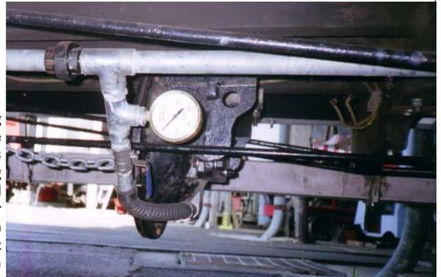
**(Above) The vacuum brake diaphragm, pipe work and gauge on underside of trailer car 93B.**
