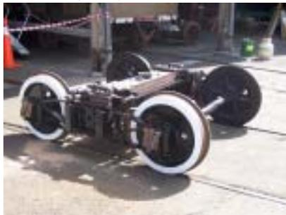
Reconditioned bogey ready for placement under 93b. New gunmetal axle box flaps and white walls complete the job. Craig tells us the original American steam tramcars were imported with white walls ??
