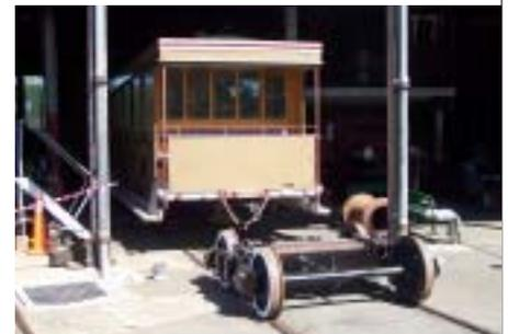
Completed bogies about to be placed under 93b.
