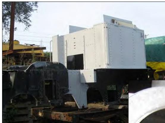
(Above) The bunker is looking much improved, sporting a new coat of primer. The interior steel plate replacement is underway.
