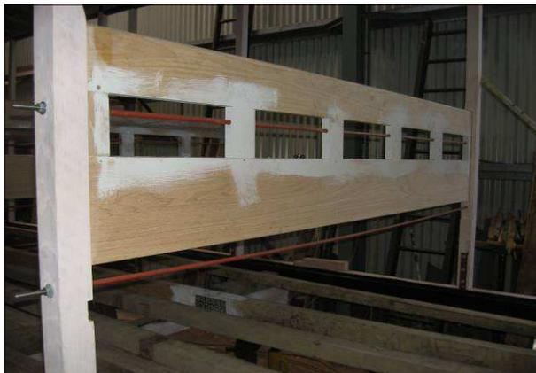
(Above) The formed seat backs and truss rods form an integral part of strengthening the car transversely.
