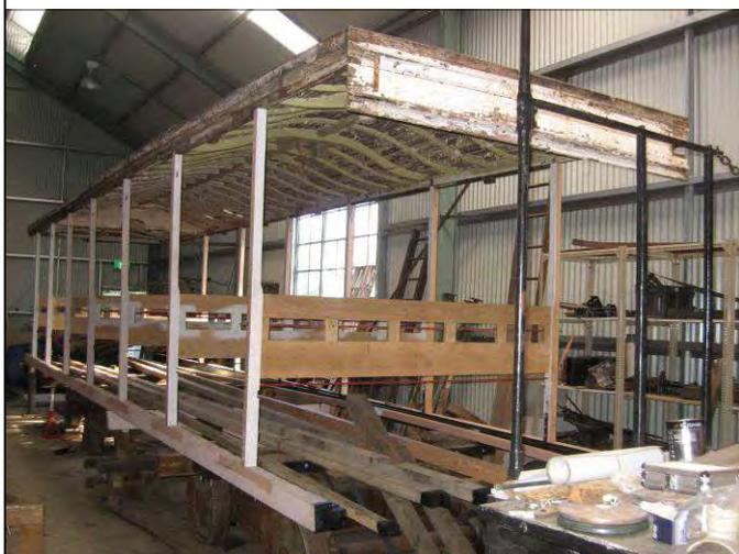
(Above) A view of 72B showing the stage just before all sub-frame timbers were fitted into the head stocks.
