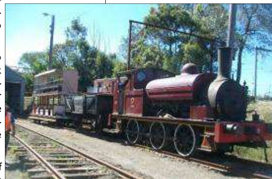
(Above) DD99 is being shunted back into the tram shed. The new end panels and solid roof on the top deck can be readily seen.
