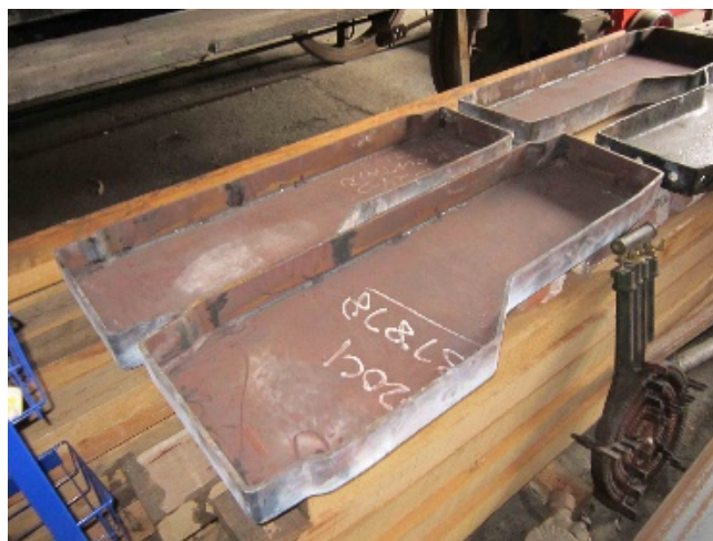
New gusset plates for 5711's tender (Photo: Ted Dickson)
