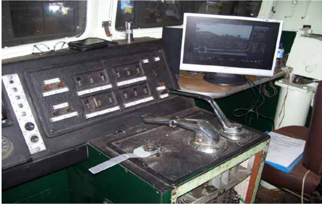
Trains Simulator Screen and Speakers in the 46 Class No. 2 End Cab. Note the replica reversing key.
