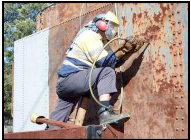
*Above: Rod Hawkes needle guns rust and loose paint from the side of 5711's tender tank. Photo: Andrew Tester.*
