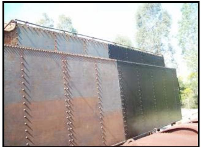
*Above: Half of one side of the 5711's tender has been treated and given its first coat of black paint. Photo: Andrew Tester.*
